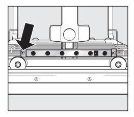
Unscrew the track with AWK (using an allen key) and remove from the retainer.
